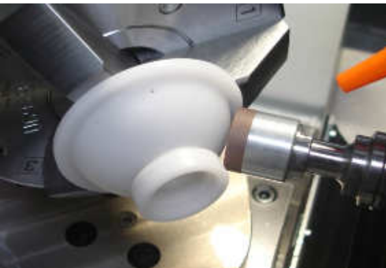
External grinding of the sphere with swivelled B-axis
