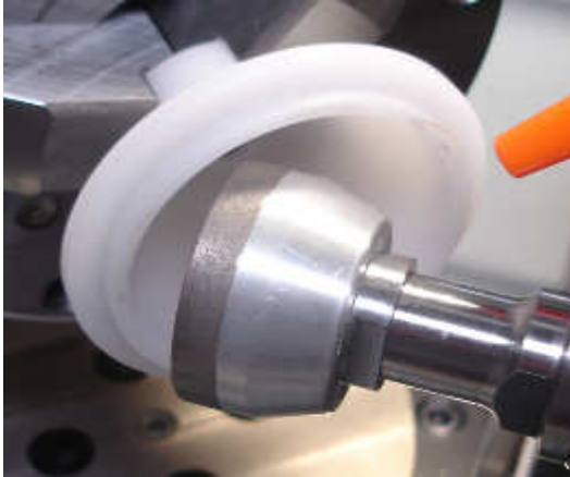
Internal grinding of the sphere with swivelled B-axis
