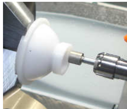
ID- and OD grinding of diameter and cone
