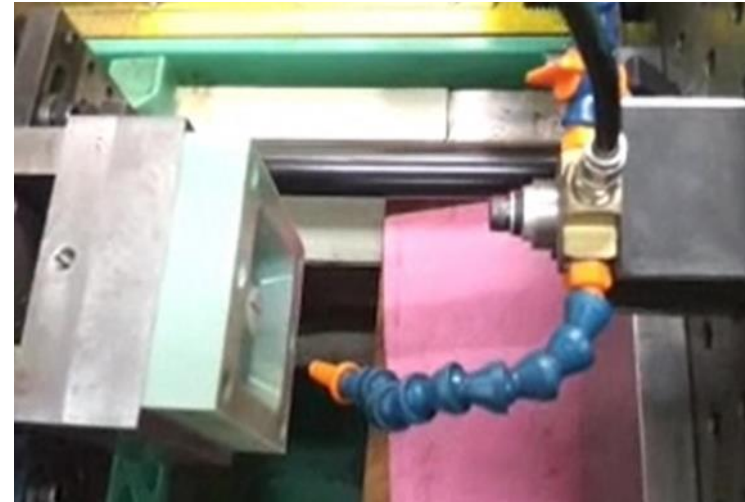
Compressed air cools mold to 50 °C (120 °F)
