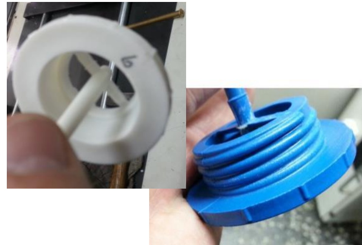
Threaded cap from mold: Left – 20% GF PP, Right- 20% GF PA 6/6
