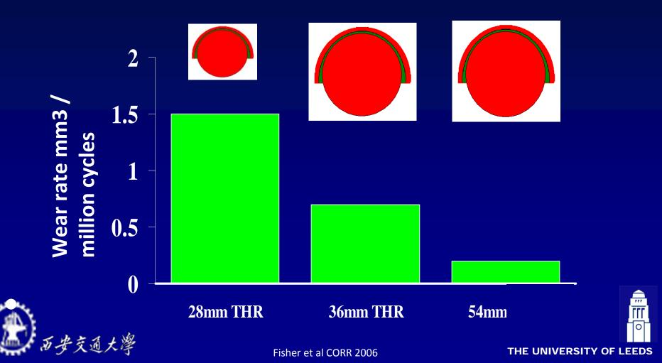
• UHMWPE hip: large diameter increases sliding distance and increases wear:
