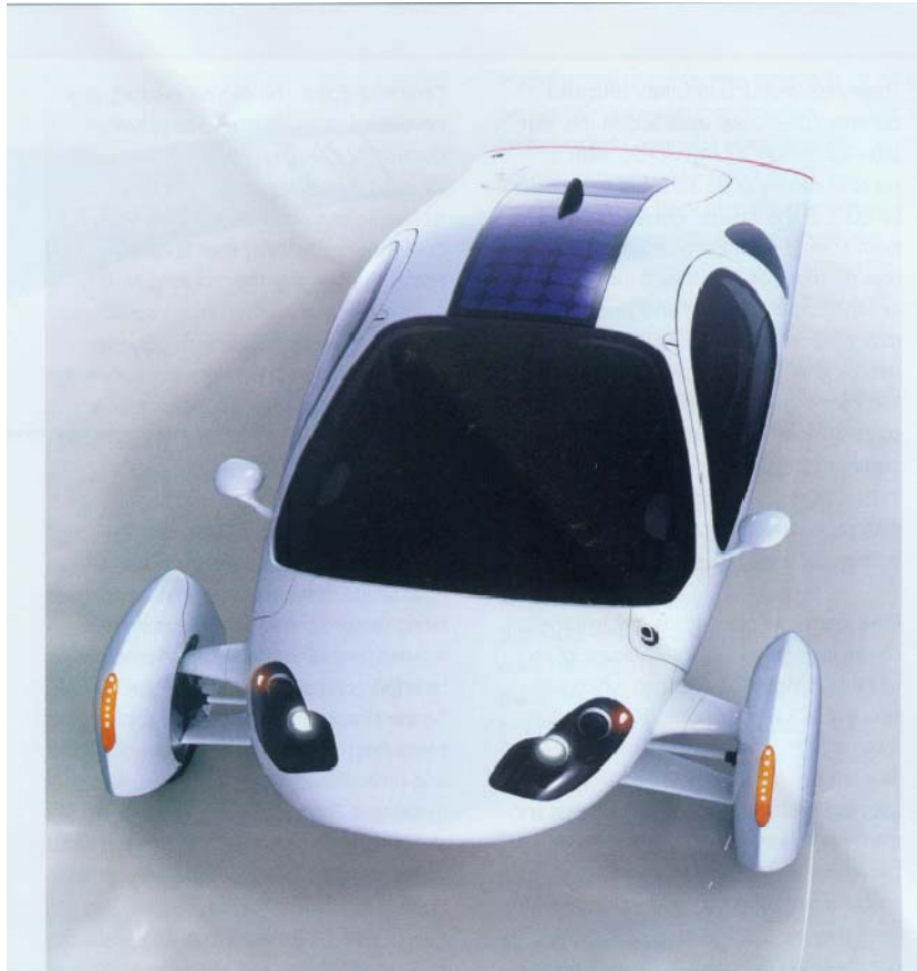
Composite body panels on the Aptera electric car make extensive use of DIAB foam core in the sandwich construction.
