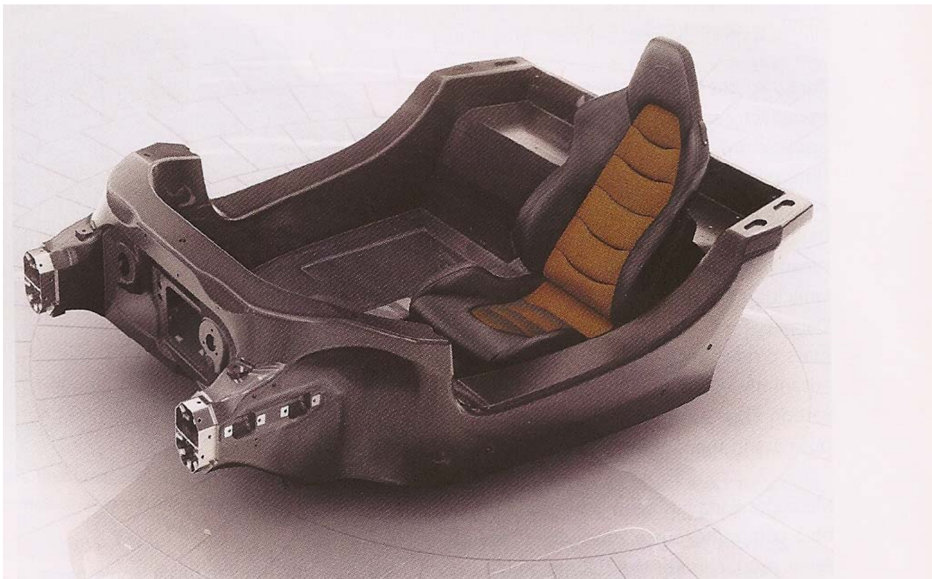
The MonoCell tub for the McLaren MP4-12C supercar is moulded as a single piece and weighs less than 80 kg (176 lbs).
