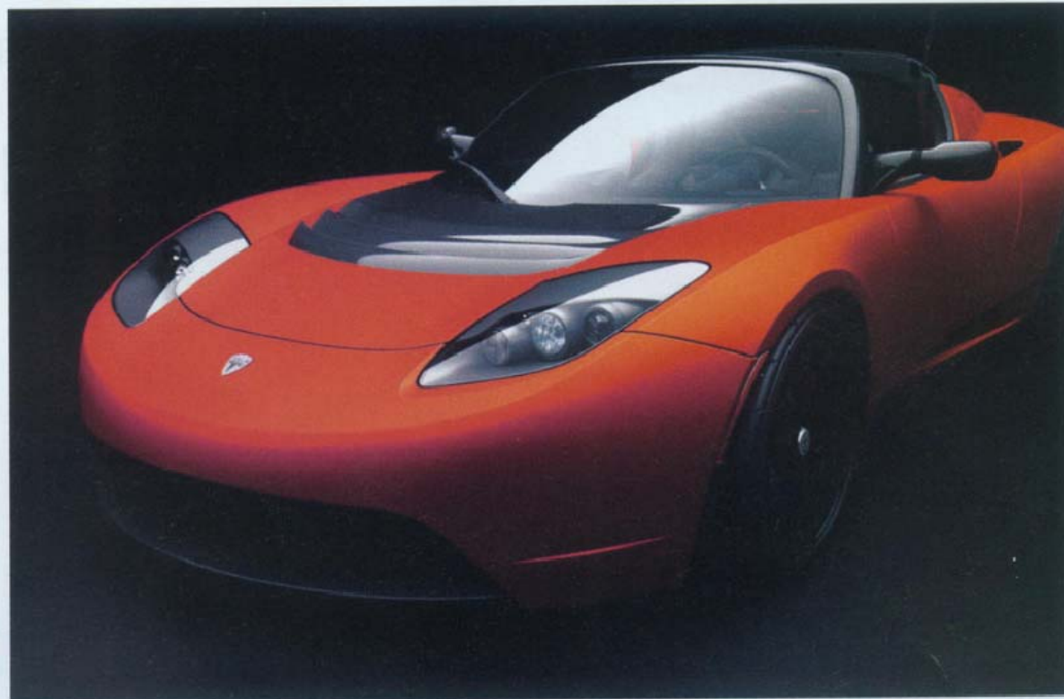
The Tesla Roadster Sport is an all-electric, high-performance sports car with innovative lightweight body panels of carbon fibre/epoxy composite.
